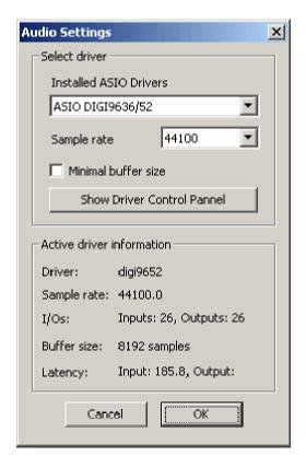
All of your installed ASIO drivers will be listed in the drop down box. From here you can open the sound cards Control panel and make adjustments to routing and sampling frequency etc. Once that is set open the Audio Routing window.
