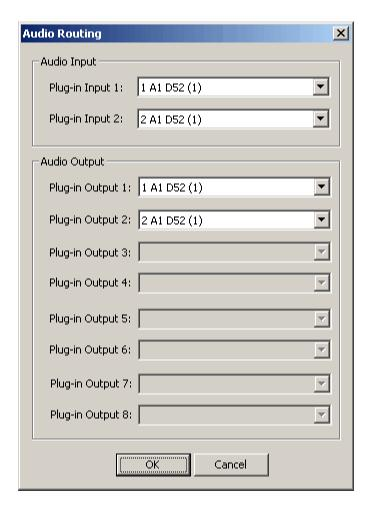
Here you can pick the stereo input and output out of all that might be available on the card. Click OK and you should hear sound coming out of the assigned output. Of course you have to feed some audio into the input first.
