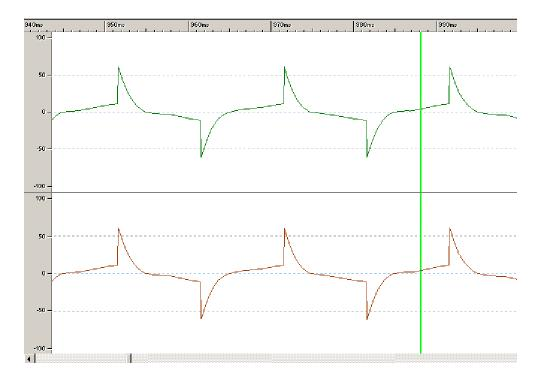
Because the speaker has little power in low frequencies it cannot deliver the pressure to keep the wave flat. The attack of each half cycle is sharp, but the sustain part decays due to limited LF ability.
